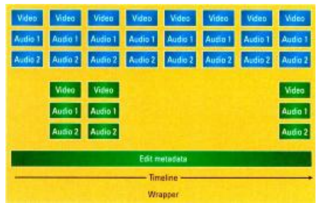
Figure 2. An AAF file could contain a base layer, a compositing layer and some editing metadata,
